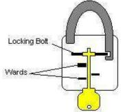
As can be seen, part of the key has been filed away preventing the key from being stopped by the ward, thus allowing the remaining end section to come into contact with the locking mechanism and open the lock.
