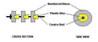
These separate parts of the lock are usually smaller plastic discs which instead of having a notch removed on its interior have a point removed on its exterior, (see above).
