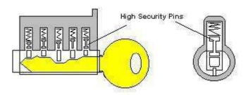
Pins of the shapes shown above increase the difficulty of picking pin tumbler locks as they give the impression, when picking the lock, that the pin has been picked. In actual fact the pin is still preventing the cylinder from turning but the recess of the high security pins allows the cylinder to turn slightly, giving the impression that particular pin has been raised to the correct height.
