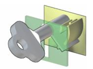
When considering how this type of lock works it is important to remember that the wards do not move in any way and are simply protrusions along the keyway to prevent any key apart from the correct key from turning inside the lock and thus moving the bolt.
