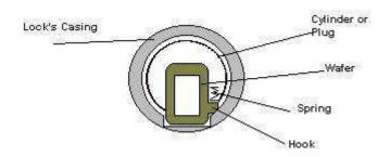
The wafers or disc tumblers are simply metal discs with a rectangular hole in the centre. Within a wafer lock there are usually around five of these discs depending on the security of the lock. When the key is inserted into a wafer lock it will pass through this rectangular hole.
