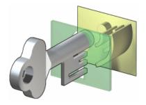
This type of lock has one or more 'wards' which prevent the incorrect key from throwing the bolt. Wards protrude inside the lock preventing a wrong key from turning and therefore from operating the bolt.
