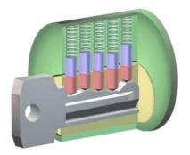
The pin tumbler lock consists of pairs of bottom pins in red, which are usually made of brass, and top drivers (in blue) constructed from steel. In the majority of locks there will be five sets of these pins and drivers.
