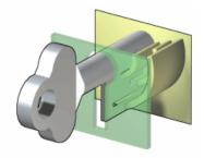
Only the correct key will open the lock due to the wards which restrict an incorrect key from turning within the lock.
