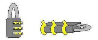
The difference between the simple bicycle lock explained above and the locks with shackles is simply that it is a section of the shackle which has the pegs on which allows the shackle to lock instead of a plug.
