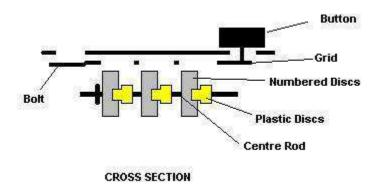
When the correct combination has been entered the metal numbered discs will in-turn rotate the plastic discs to the point at which a part has been removed.
