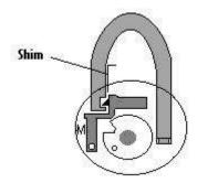
With the non snap-closed lock once the dial has been rotated in the correct sequence and the shackle is open, if the dial were to be turned with that shackle still in the unlocked position then the lock would be unable to be locked as the bolt would not spring back.
