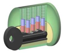
Many high security locks use mushroom or spool pins in order to make picking this type of lock much harder. This can be shown from the diagram below.
