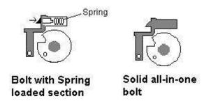
as the Many of these combination dial locks have a circular body and therefore allow easy access to the spring loaded bolt.
