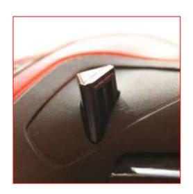
that the drive mechanism moves in is not relevant because either way the mechanism will still go up and down. It is important to ensure that the direction switch is fully pushed either to the left or right because if you have it in the middle the gun will not operate.
