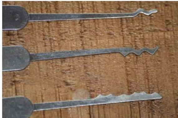
These picks are designed for raking locks. Their purpose is to rapidly vibrate the pins within the lock.
